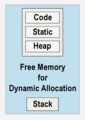
This is called a virtual address space layout, which is divided into four categories of storage shown as code, static, heap and stack
