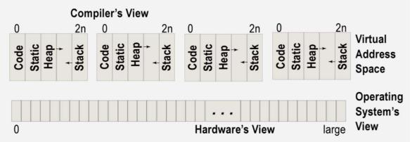
"The heap and the stack grow toward each other...From the compiler's perspective, this virtual address space is the whole picture. However, modern computer systems typically execute multiple programs in an interleaved fashion. The operating system maps multiple virtual address spaces into a single physical address space supported by the processor." pp 254-255
